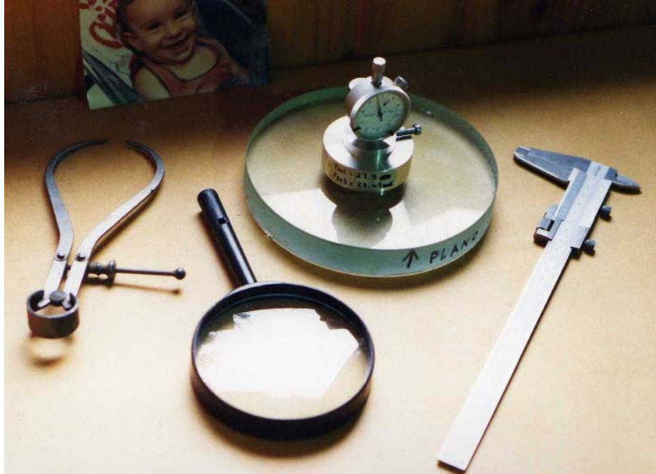
Fig 25. The lens and the elements needed to define it by the prescription below. Lacking a refractometer it was assumed the glass is BK7 (System 2-lupach)
